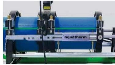
Welding of the aquatherm electrofusion sockets is only allowed at a temperature between +5°C and +40°C (according to DVS 2207). Make sure that the aquatherm electrofusion sockets and the, to be welded, pipe ends are 100% dry (i.e. free from condensation).
