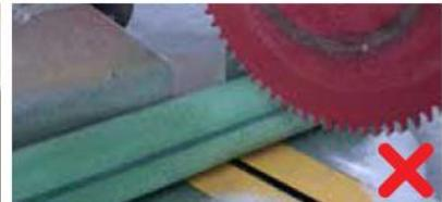
Don't use power cutters if the pipe is 40 °F or colder. Cold pipe can crack and split. Warm the pipe before cutting it.
