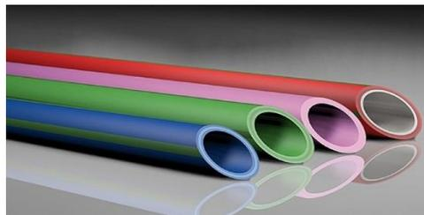
For the application in open air aquatherm offers composite **aquatherm green pipes** and **aquatherm blue pipes** with an UV-protective layer made from **black polyethylene** (PE with carbon black), which excludes damage caused by sunlight. This PE layer must be peeled off, prior to welding.
