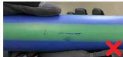
Don't use damaged pipe that is gouged deeper than 10% of the wall thickness on the outside or 5% on the inside.
