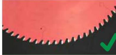
Use a circular hardwood blade (60-100T) with carbide teeth. This will produce a cut that needs little to no clean-up.
