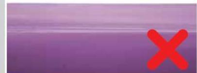
White stress marks and cracks indicate damage. Reassess any cutting tools that leave cracks. You may need to squeeze the end of the pipe to see small cracks.
