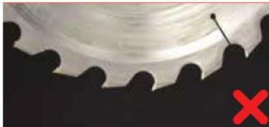
A wide-toothed blade (24-40T) will produce a jagged cut that is rough and not desirable for socket fusion.
