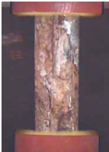
► Corroding steel pipe
