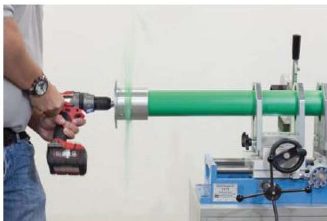
▲ Universal peeling tool (here: 75mm, Art.-No. 50485) and extension (here: 75mm, Art.-No. 50495)
