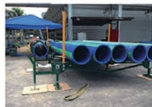
In addition to offering the installer a system much lighter than metal, Aquatherm Blue Pipe also provided the University of Florida with a rust- and corrosion-resistant chilled water piping option.
