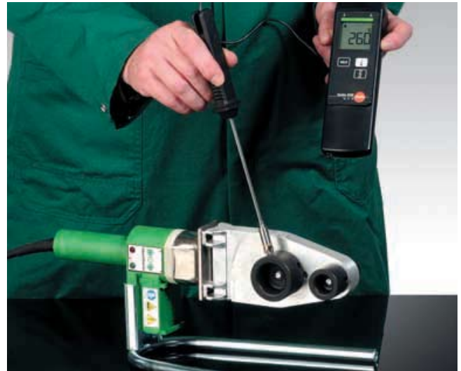
Temperature control with a thermometer
