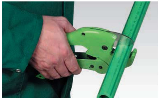
Cutting of the pipe
